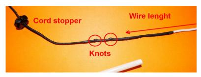
After the element wires are cut to the right length and have been fed into the brass crosses, they are connected with the 2 mm rubber cords. This is done by placing 2 small and very tight knots in the rubber cord and shrinking a 10 cm piece of 2 mm shrink tubing onto the wire and the rubber cord with the knots. The knots prevent the cord from slipping out of the shrink tubing. Rubber cord length should be around 30
