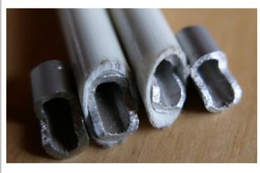
The 45 ° cuts at the boom intersections are not a perfect axial winding protection. Sometimes it needs some manual alignment by hand after setting up the antenna to make the elements being perfectly parallel. This can be improved by small inserts made of 6 mm aluminum tubes.
