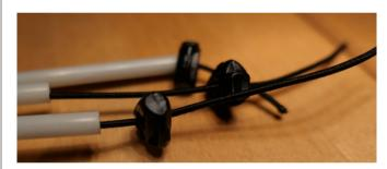
The last step is to feed the element rubber cord and wires through the fiberglass tubes. As final step, put the cord stoppers on the rubber cords in order to lock the elements onto the boom.
