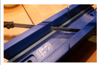
Fiberglass pipes are really a robust material, but some care has to be taken when cutting them. The ends tend to fan out. Use a hacksaw with fine teeth and a cutting jig as shown if possible. The cutting jig also helps to make the accurate 45 ° cuts in order to secure the boom against winding.
