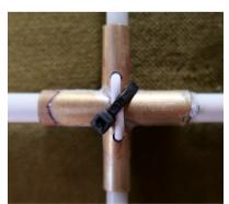
Cut wires of appx. 1 m. Feed one end through the left hole, one end through the right hole. Repeat this for all elements left. Fixate the wires with a cable tie as shown in the picture.
