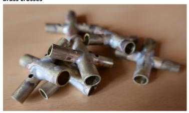
Manufacturing the 6 crosses out of brass tubes is the most time consuming part of building this antenna and will challenge your patience. The trick is to hard-solder the two pipes orthogonally together. Otherwise your Yagi antenna will look strange!
