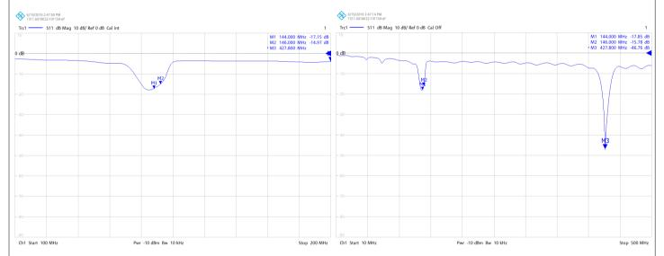
The two plots show the return loss of my second prototype antenna. I built this antenna with the element length shown in the table above which are based on simulation. Resonance is appx. 2 MHz too low but this not a real problem as the electrical design is of quite wide bandwidth.
